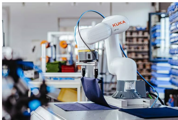
Figure 2. Small robot grabbing fabric, Kuka [11]
