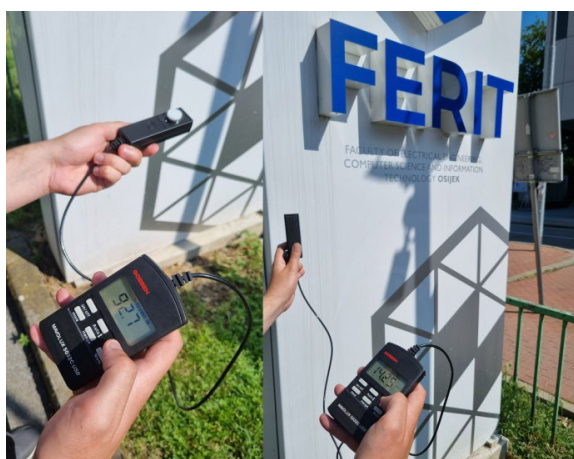
Figure 5. Illumination and luminance at the second point of measurement
