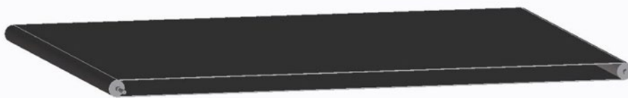
Figure 4. Belt between rotating rollers
