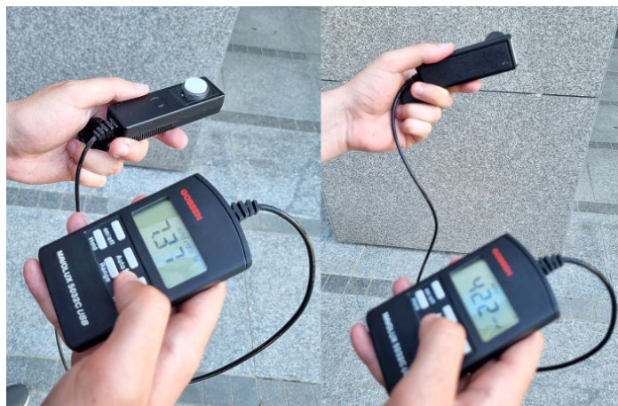
Figure 4. Illumination and luminance at the first point of measurement
