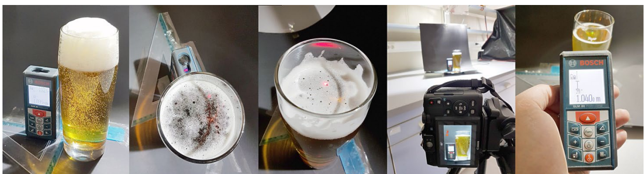
Figure 3. Determining the stability of beer foam with a laser rangefinder [8]
