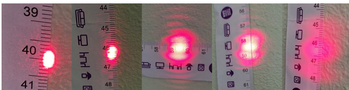
Figure 6. Increase of laser beam surface concerning distance
