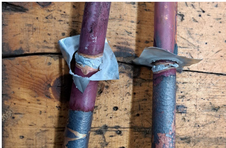
Figure 3. Failed furnace brazing attempt
