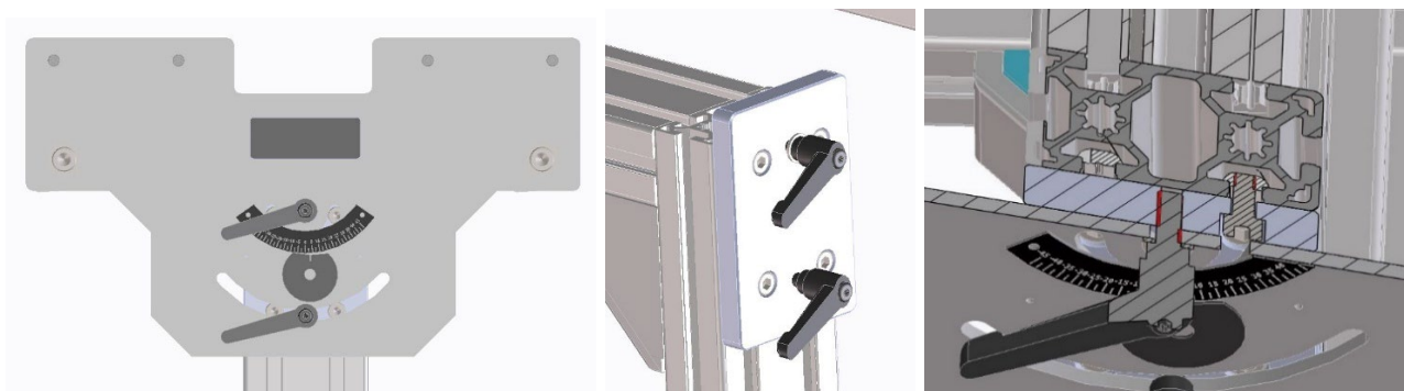
Figure 13. Working principle of angle regulation
