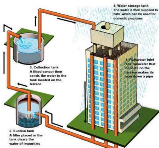
b. above-ground placement of rainwater tanks
