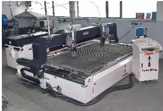
Figure 5. Used machine for waterjet cutting - TENKING 23020
