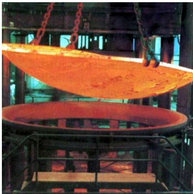
Figure 4. Heated and formed segment of spherical tank
