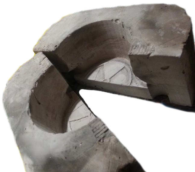
Figure 3. Plaster mould after PLA melting
