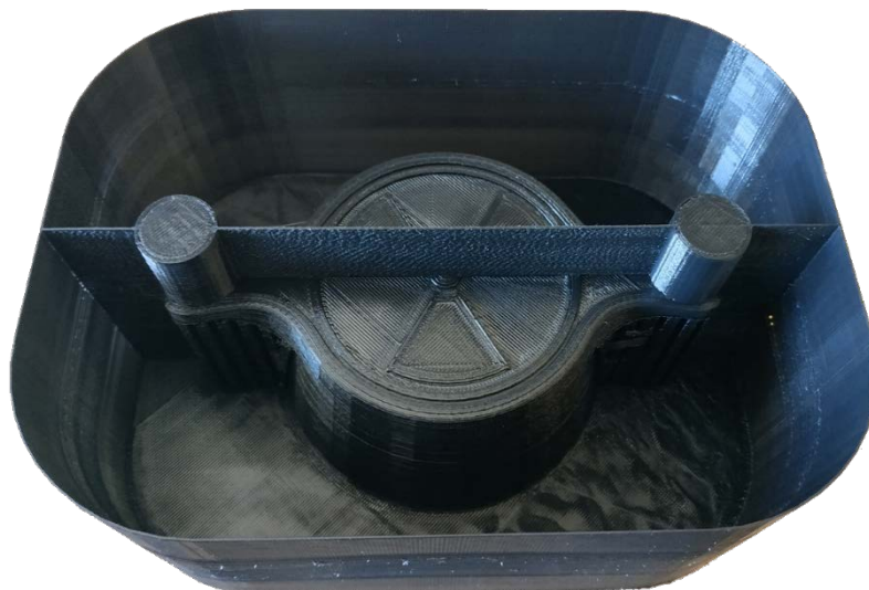
Figure 2. The PLA mould for plaster mould
