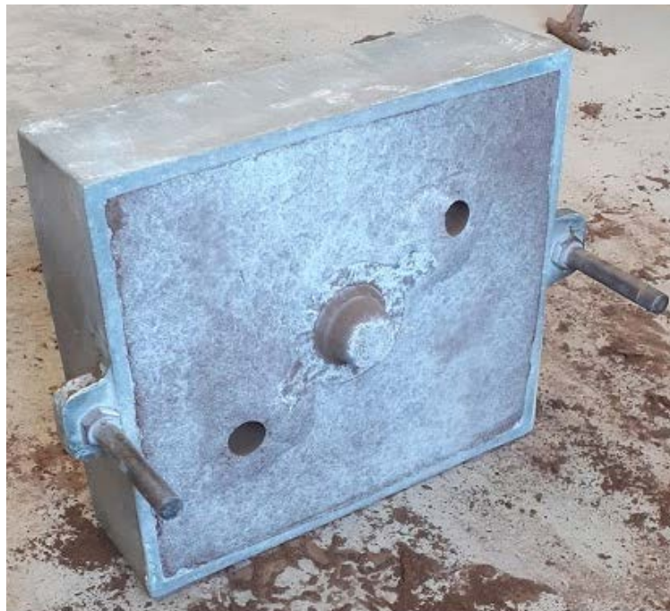
Figure 7. Cope with core, runner and riser
