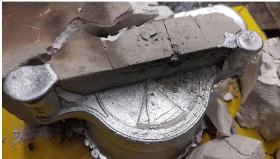
Figure 4. Storage crucible after plaster mould casting
