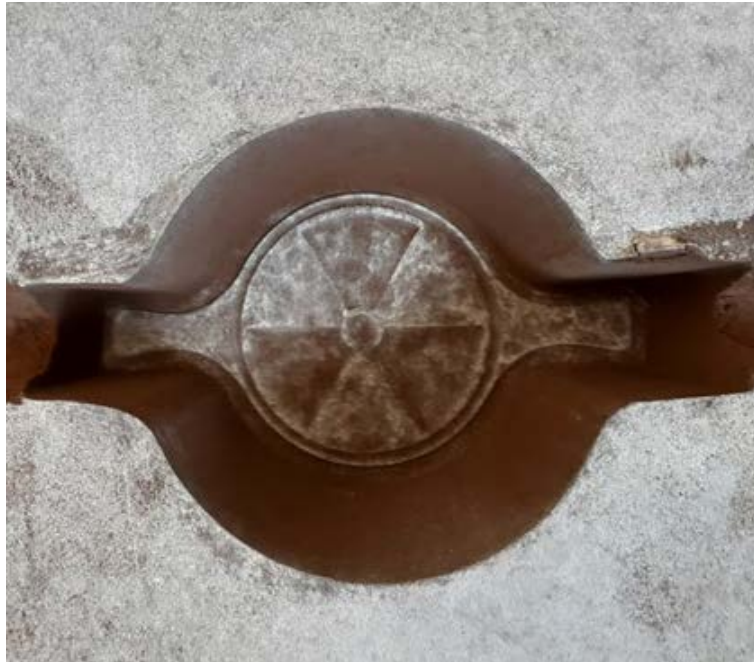
Figure 6. Mould cavity in the Drag
