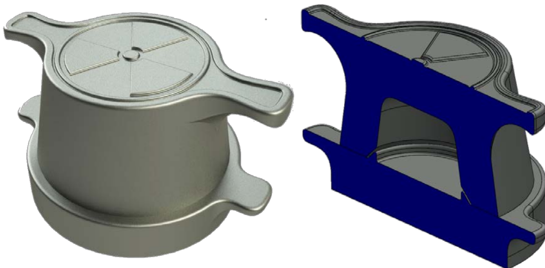
Figure 1. CAD model of the lead crucible
